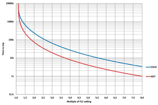
Fig. 11 RSGD Class 10 motor overload trip profile
