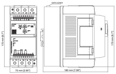
Fig. 3 RSGD..55..VX310C to RSGD..85..VX310C (DIN rail mount version)
