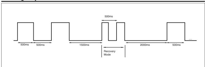
Note: During recovery from an alarm condition, the red LED will flash at twice the normal flashing frequency between successive flashing cycles as shown above to indicate that the softstarter is in recovery mode which recovery lasts for 5 minutes
