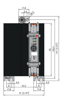
Housing width tolerance +0.5mm, -0mm as per DIN 43880. All other tolerances +/- 0.5mm. Dimensions in mm.
