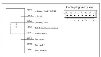
\* Active high: ON > 9 VAC/DC, OFF < 6 VAC/DC Active low: ON < 6 VAC/DC, OFF > 9 VAC/DC
