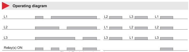
Fig. 1 Total phase loss, phase sequence
